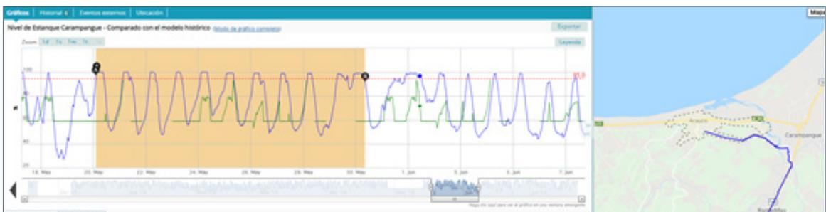
TaKaDu found that every night the tank was losing at least 3 l/s for six hours. Essbio-Nuevosur has since acted to reverse this situation, modifying the way the pumps are operating.
